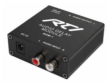
The ADM-1 Audio Delay Module is the ideal problem solver to lip-sync issues between audio output devices. For instance, when a television's internal speakers and ceiling speakers wired to an external audio system are used at the same time, there may be a noticeable delay due to differences in audio processing speed. The ADM-1 makes it easy to compensate for this delay and get the sound back in sync.
